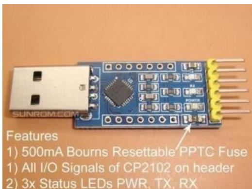
UART stands for universal asynchronous receiver/transmitter and defines a protocol, or set of rules, for exchanging serial data between two devices. UART is very simple and only uses two wires between transmitter and receiver to transmit and receive in both directions. Both ends also have a ground connection.
