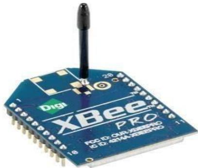
Zigbee is a wireless network module that is being controlled globally. It is a low power network and comprise of sensors, control systems and instrumentations. Its benefits are really beneficial for domestic purposes and they can be seen in medical monitoring, industrial automation, low power network and comprise of sensors, control systems, instrumentation and HVAC Control.
