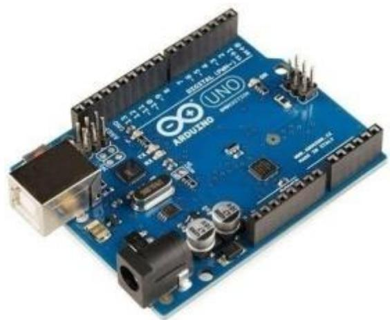
Arduino UNO is a low-cost, flexible, and easy-to-use programmable open-source microcontroller board that can be integrated into a variety of electronic projects. This board can be interfaced with other Arduino boards, Arduino shields, Raspberry Pi boards can control relays, LEDs, servos and motors as an output.
