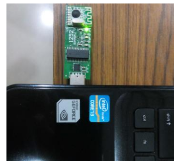
Figure15. RF receiver attached to PC receiving the signal from RF Transmitter
