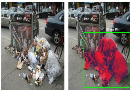
Figure 8: Left - input image showing garbage, Right - coarsely segmented output image
