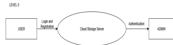
Figure 2. Level 0 Data Flow Diagram
