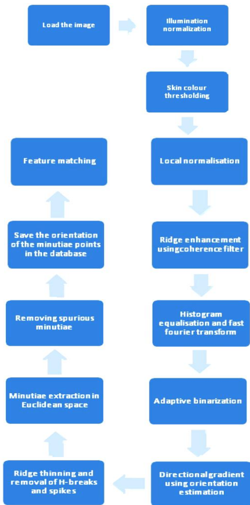
Fig.2.1 Block Diagram of Present System
