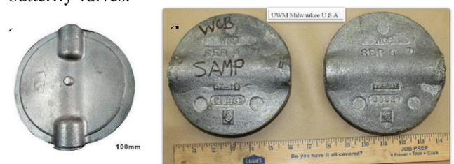
Figure 3. (a) A commercially available butterfly valve, (b) surface alloyed butterfly valve prototypes cast at the industrial foundry and UWM
